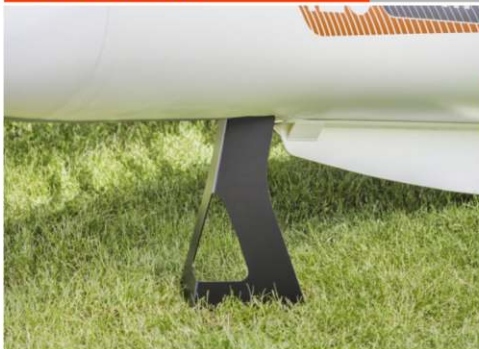
Pair , aluminium alloy ; Weight: 1,9 kg
